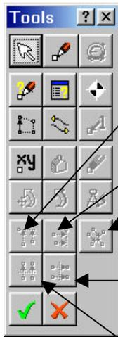
Used to align horizontally the selected control points. After pressing the button the cursor changes to a question mark at which point you should point and click near a selected control point. All selected control points are then aligned horizontally with this point.
