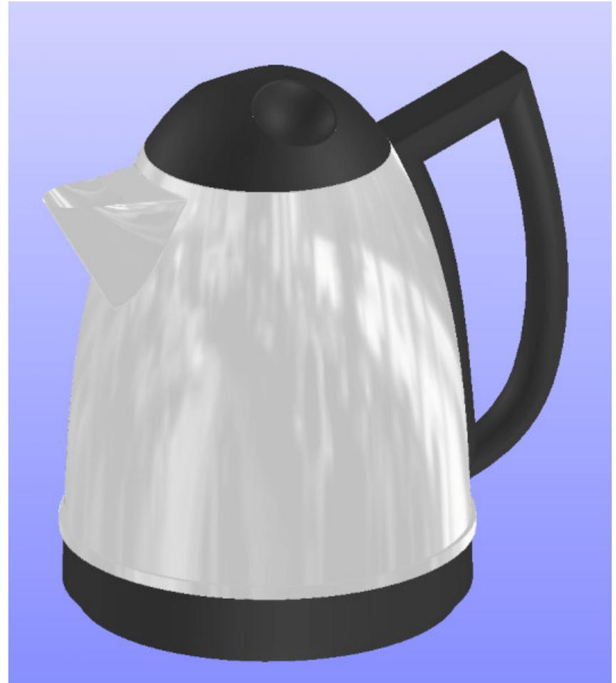
Many of the parts in this model are clearly going to be modeled separately. The body and the spout although both chrome material need to be made independently because their shapes are so different.
