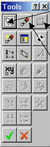
Sets the editing mode to point selection. This is indicated by an arrow cursor. In this mode points can be selected. Multiple Selection can be achieved by the SHIFT key. Once selected these points can be moved, scaled (CONTROL key) or rotated (SHIFT key). The right mouse button reverts to edit mode.
